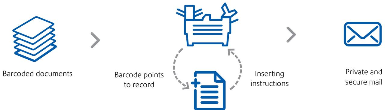
The reference file is used to control and constantly verify pages that are accurately folded and inserted.
